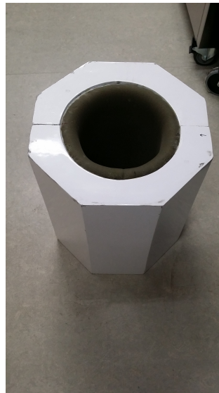
(b) Coil B, prototype Mregen coil system; cavity large enough to rest appendage during PEMF exposure treatment.
